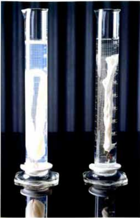
The Draves Wetting Test (left) predicts how thoroughly and rapidly an adjuvant will wet and penetrate plant tissue by measuring how thoroughly the solution wets cotton skeins.
