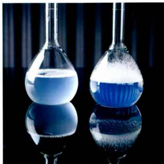
Anti-Foam agents are added to a tank before other solutions to prevent the formation of foam.
